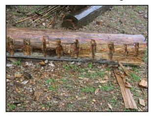
2. Then the logs would be scraped down to the notches to get a squared log.
